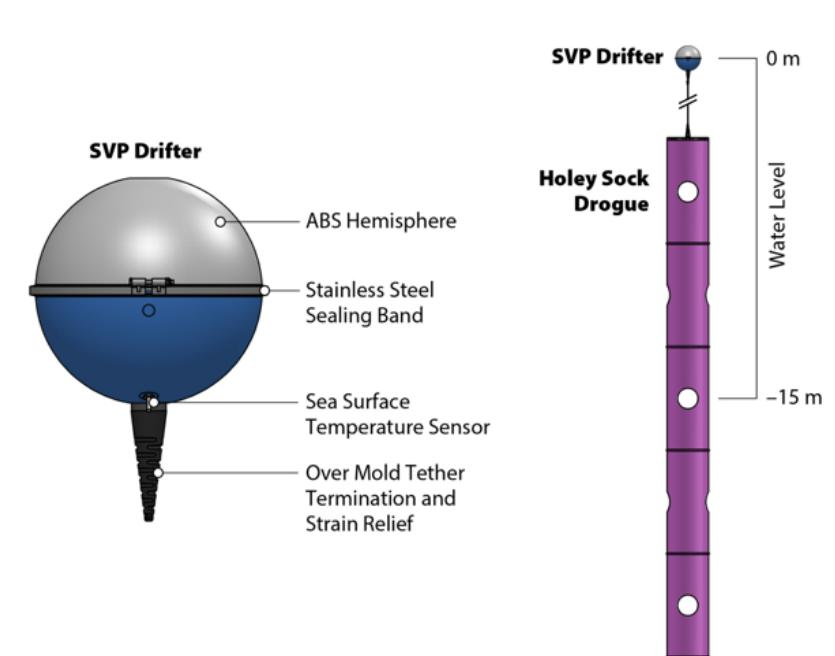
SVP drifters with drogue at 15 m depth are the primary source of in-situ global observations of near-surface ocean currents and have been used for decades to study the ocean circulation and dynamics from sub-mesoscales ( $\sim 1$  km) to basin scales (1000 km) (Niiler et al., 2001; Centurioni, 2018)
